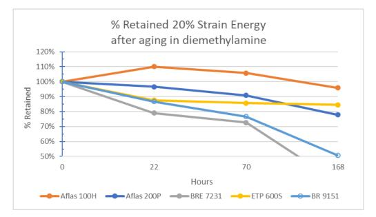
Figure 2: Percent Retained Strain Energy Density after aging
