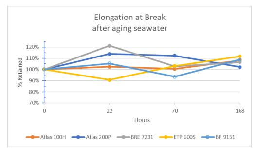
Figure 11: % Retained Elongation at Break after aging
