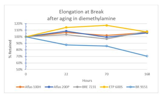
Figure 5 - Percent Retained Elongation at Break after aging
