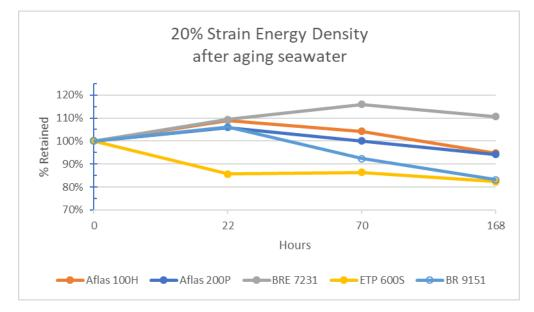
Figure 8: % Retained Strain Energy Density after aging
