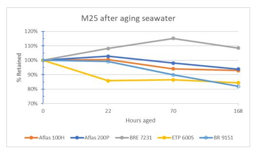
Figure 9: % Retained M25 after aging
