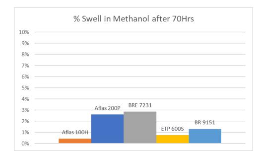
Volume change in both solvents was conducted at room temperature (22C), fully immersed. Volume change was calculated per ASTM D471-16 sections 12 and 18.
