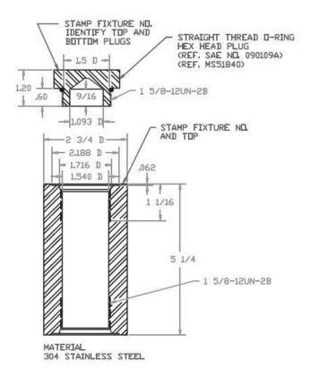
Figure 1: Seawater aging vessel
