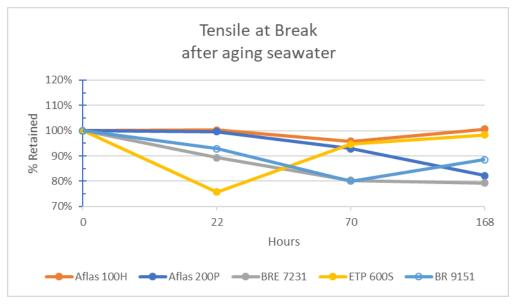
Figure 10: % Retained Tensile at Break after aging
