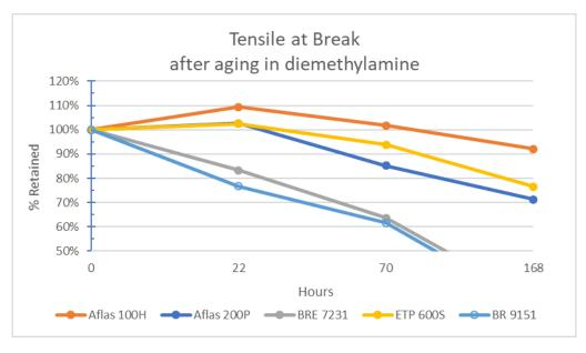
Figure 4: Percent Retained Tensile at Break after aging
